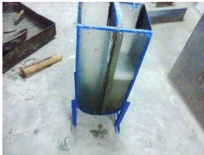
Fig: 4 U-Box Test
