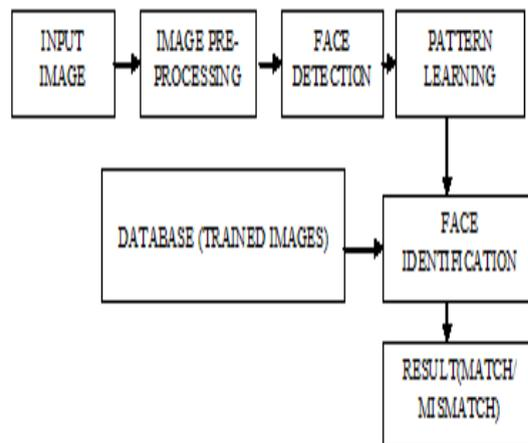
Fig. 1. Block diagram for face recognition process
